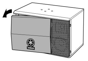
**3.** Remove the 4 screws that hold the metal speaker grille.
